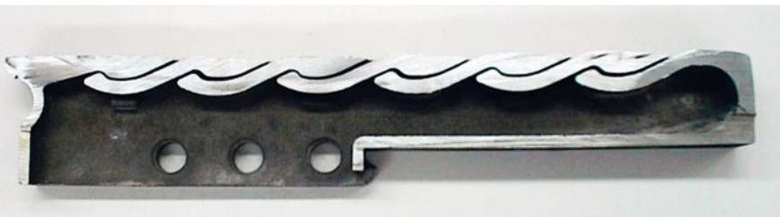
**4** Cross section of a slotted plate (Coanda Nozzle) of the KIDS range
