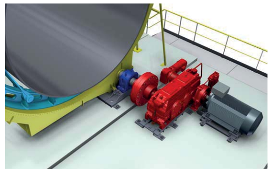
IKN kiln drive
