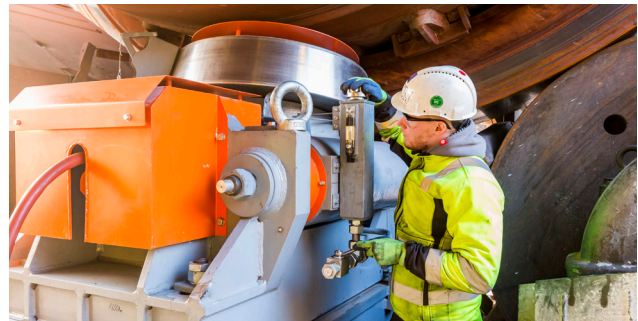
Hydraulic thrust unit inspection
